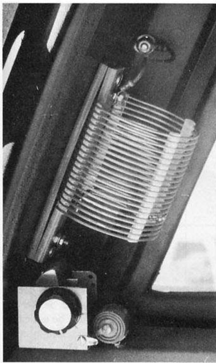
Fig 2—A view from inside the vehicle shows the 40-meter loading coil, shunt capacitors (below the coil), mounting bracket and antenna.
